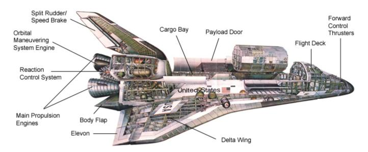
The airplane-like control surfaces on the orbiter are useless in the vacuum of space. However, once the orbiter re-enters the Earth's atmosphere, these control surfaces interact with the air molecules and their airflow to control the orbiter's flight path.
